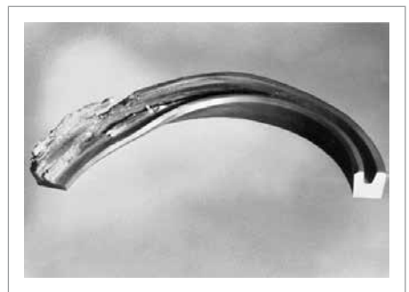
Fig. 18 U-ring destroyed by hydrodynamic pressure build-up
