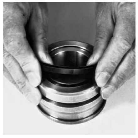
Fig. 43 Snapping in the polyurethane running ring
