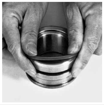
Fig. 44 Snapping in the polyurethane running ring
