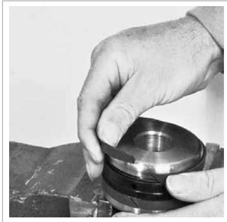
Fig. 49 Snapping in the guide back-up ring
